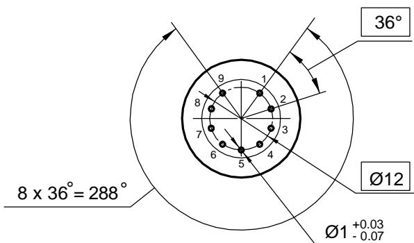
Electrode -to - lead connection diagram
