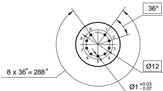
Electrode -to - lead connection diagram
